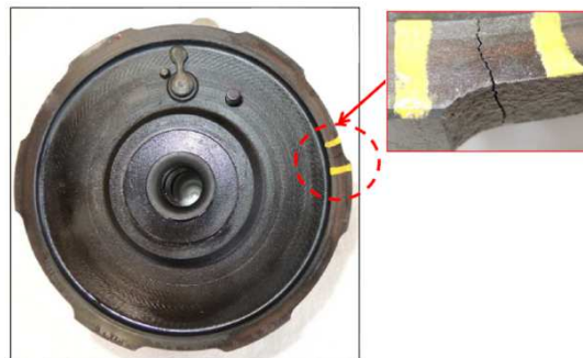
Fig. 2. Breakage of the flange of bearing housing
