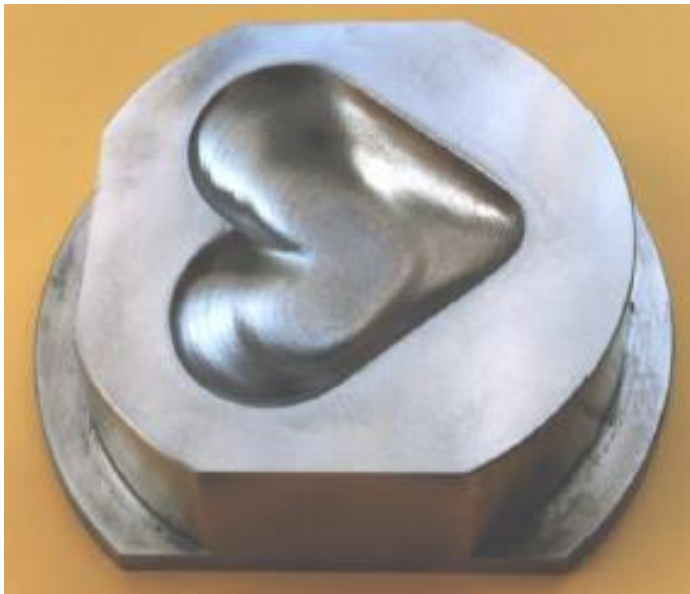
Fig.13. Workpiece after electrochemical smoothing (surface after rough milling with ball ended electrode ( R = 9 mm), time of finishing t = 45 min; other parameters: U = 16 V, v_p = 42 mm/min, S_0 = 0.2 mm, electrolyte – 15% water solution of \text{NaNO}_3 , the initial waviness after milling D = 0.1 mm; the final waviness after ECM smoothing \approx 0,0 ; R_a \approx 2 \mu\text{m} ; based on [6, 19])
