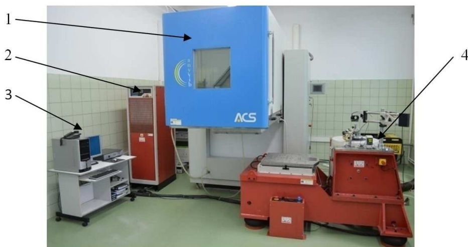
Fig. 1. Test stand for conducting fatigue tests
