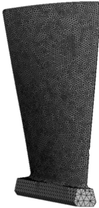
Fig. 2. Blade discrete model
