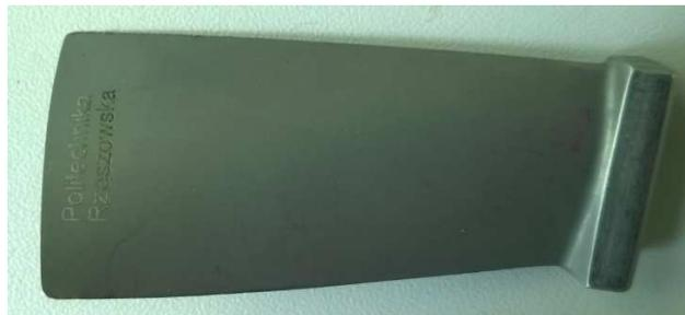
Fig. 4. 1<sup>st</sup> stage aircraft engine compressor blade
