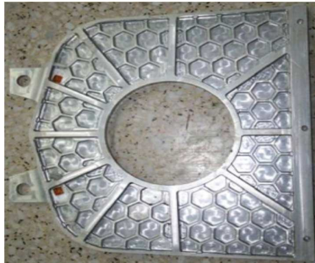
Fig. 9. A new bionic model of an aircraft reinforce frame produced by CNC milling, based on [5]
