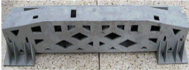
Fig. 8. A new bionic model of aircraft crossbeam fabricated by investment casting, based on [5]
