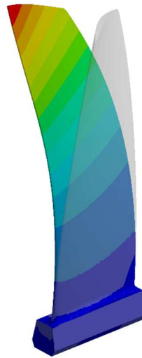
Fig. 2. Modal analysis of a blade
