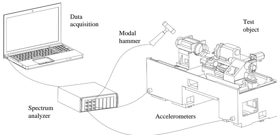
Fig. 4. Experimental setup
