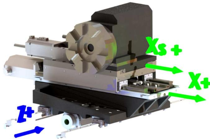
Fig. 2. Feed drive system details
