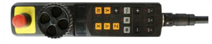
Fig. 1. Remote control used in milling machine
