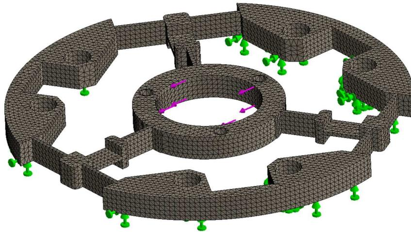
Fig. 4. Discretization of the six-axis sensor with
