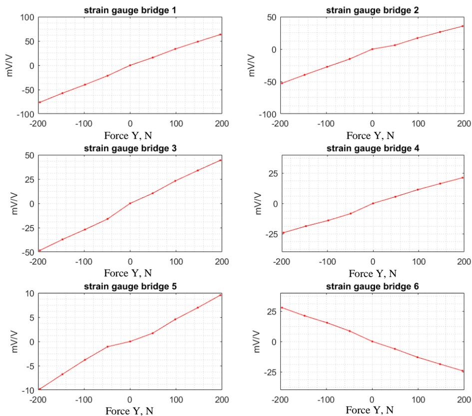
Fig. 9. Result of measured tensometric bridge voltage as a function of loading force in Y direction
