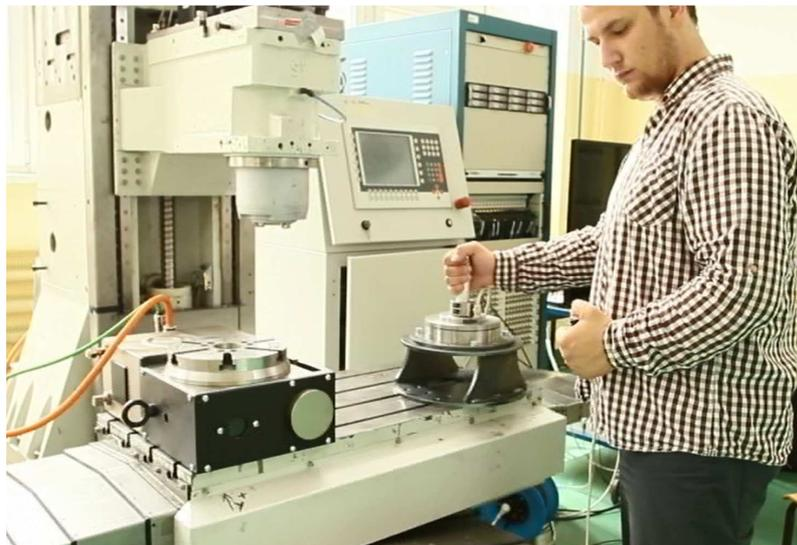
Fig. 10 Designed joystick connected to CNC machine during functional test performed by operator
