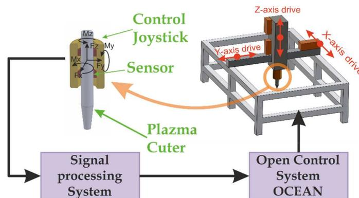
Fig. 2. Scheme of control unit with six-axis joystick
