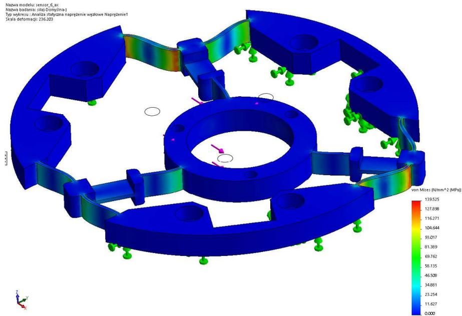
Fig. 5. The distribution of stresses with force load  $-150\text{ N}$  on direction X
