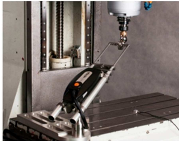
Fig. 1. Laser tracer used to determine Volumetric Error vector field
