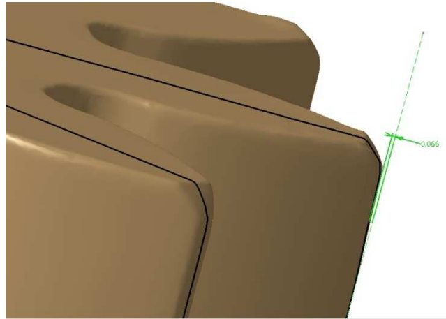
Fig. 9. Distortion of tooth surface as wiping (0,066 mm)
