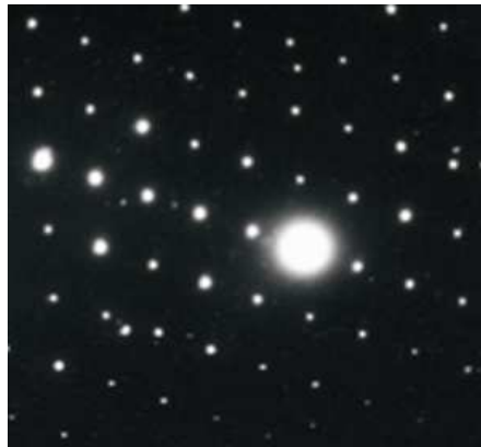
Fig. 5. TEM micrograph of AlCu 4 Ni 2 Mg 2 alloy showing the precipitate of the S-Al 2 CuMg phase (a), and corresponding electron diffraction pattern (b, c)
