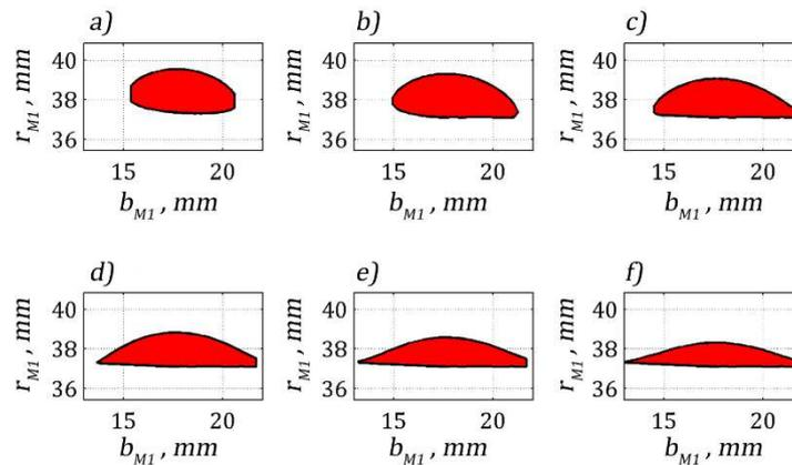
Fig. 1. The influence of axes distance error on contact pattern of cylindrical external Novikov gear: a)  $\Delta a_x = 0$ , b)  $\Delta a_x = 0,01$  mm, c)  $\Delta a_x = 0,02$  mm, d)  $\Delta a_x = 0,03$  mm, e)  $\Delta a_x = 0,04$  mm, f)  $\Delta a_x = 0,05$  mm [11]
