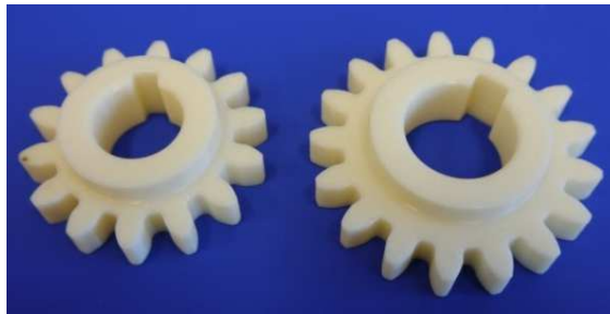
Fig. 7. A pair of gears formed in FDM technique – a nominal model
