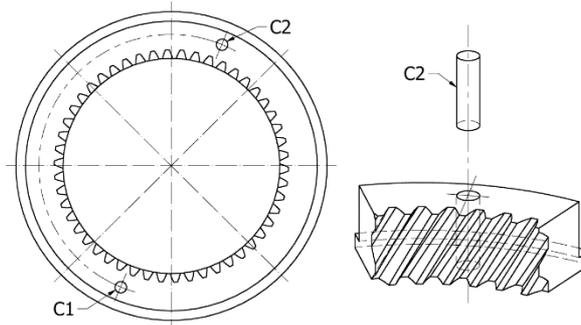
Fig. 1. Ring gear made of AISI 9310 low alloy steel – used for preparation of specimens for thermal properties investigation
