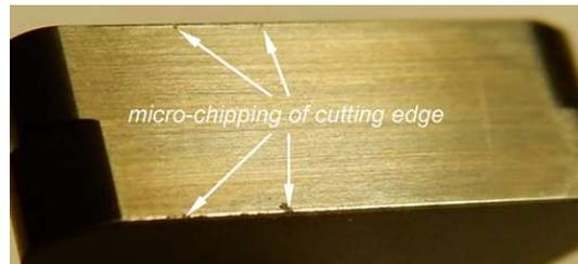
Fig. 5. Characteristic cutting edge micro-chipping of CBN inserts
