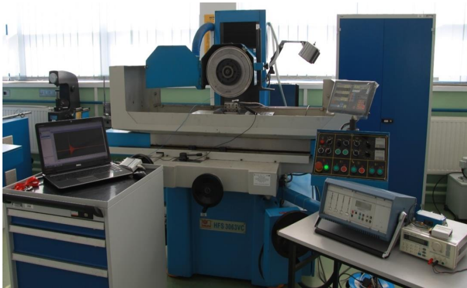
Fig. 1. Metal-working equipment for friction hardening flat surface
