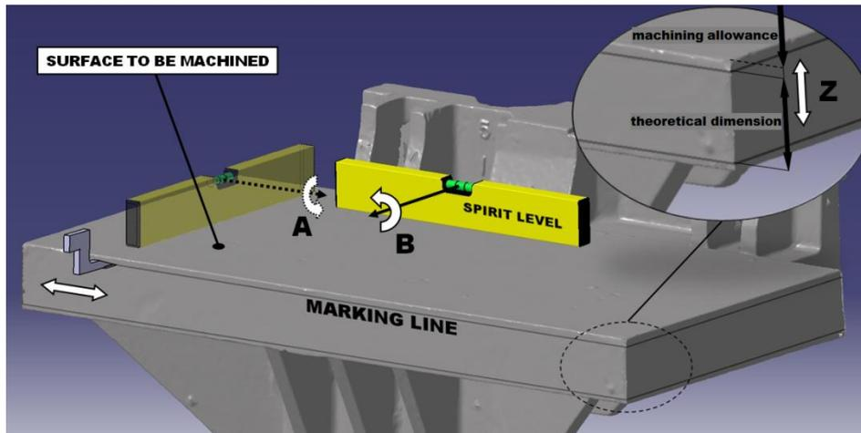
Fig. 1. Layout process
