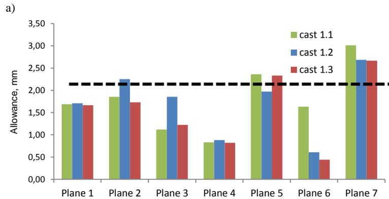
Fig. 9. The minimized allowances distribution for the series of research pieces (dashed line – minimal allowance according to ISO 8062:1997) for casts: a) 1.1,
