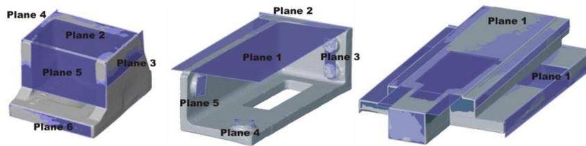
Fig. 8. Analyzed planes of measured casts
