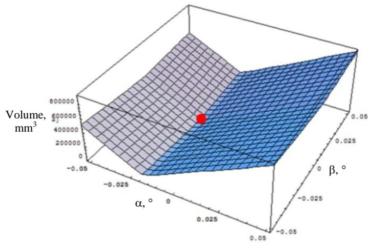
Fig. 7. The predicted volume of removed material of cast 2.1 for the minimized value of rotational displacement around Z axis of machine tool
