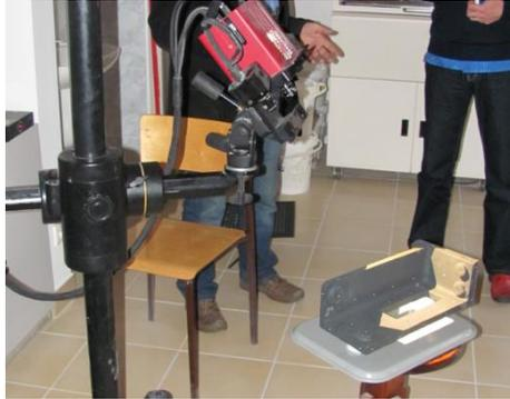
Fig. 4. Measured cast with reference elements of optical system
