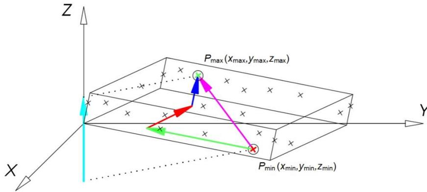
Fig. 3. Minimal machining allowance as sum of three vectors projected onto normal  $Z$ -axis
