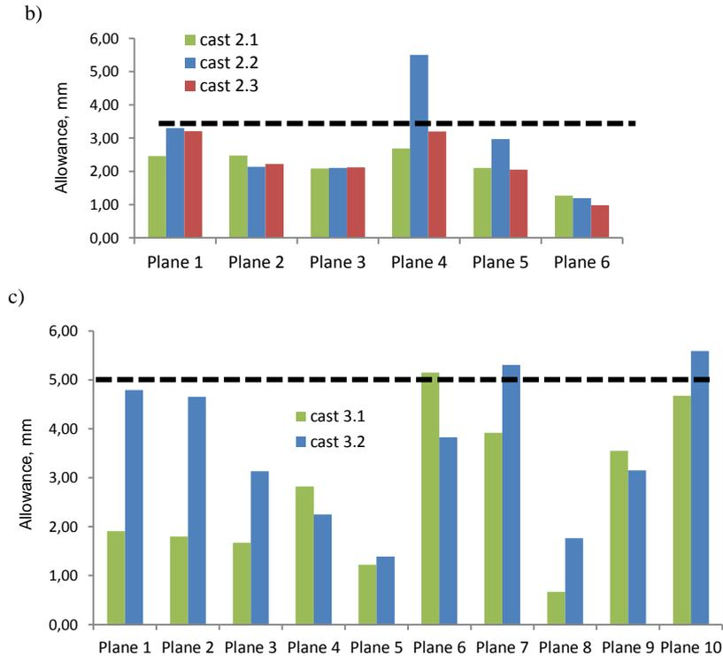
Fig. 9. The minimized allowances distribution for the series of research pieces (dashed line – minimal allowance according to ISO 8062:1997) for casts: b) 2.1, 2.2, 2.3, c) 3.1, 3.2
