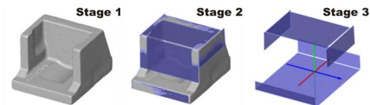
Fig. 5. The process of measurement: stage 1 – capturing coordinates of the cloud of points constituting the cast, stage 2 – substituting the selected surfaces by planes, stage 3 – introducing initial local coordinate system
