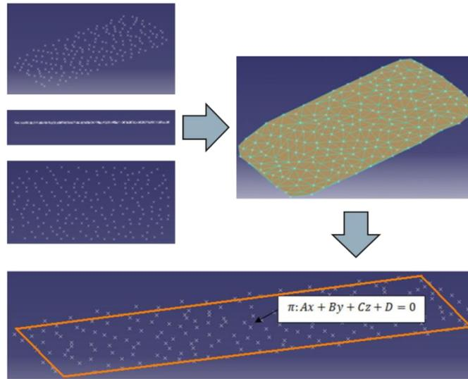
Fig. 2. Measured cloud of points substituted with nominal plane
