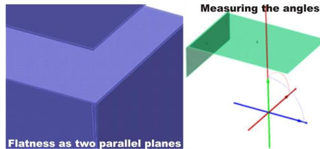
Fig. 6. Introducing the plane characterizing the machining surfaces and measuring the angles between the plane and respective axis and the flatness
