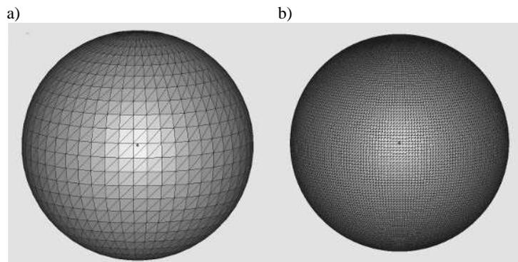
Fig. 1. STL representation of rough (a) and smooth (b) surface of sphere
