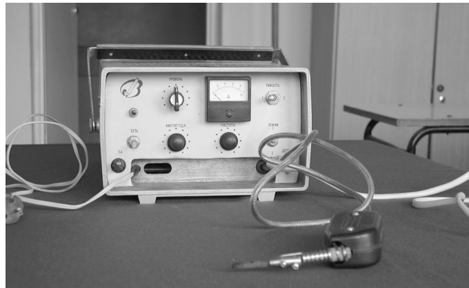
Fig. 1. View of EIL-8A – electro-spark deposition equipment
